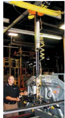
Torque tube with integrated vacuum handling device
